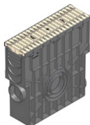
Trash box with PE mud bucket and FIBRETEC design slotted grating in the colour Sand SW 9 mm, class C 250, locked
