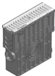
Trash box with PE mud bucket and slotted grating SW 80/10 mm, class A 15, locked
